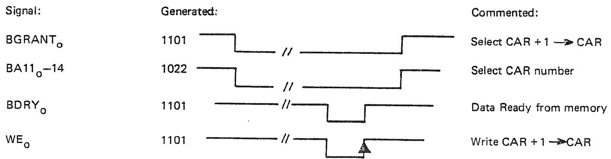
Figure 6.5: LOAD MPX-CAR (IOX LOAD CAR)
