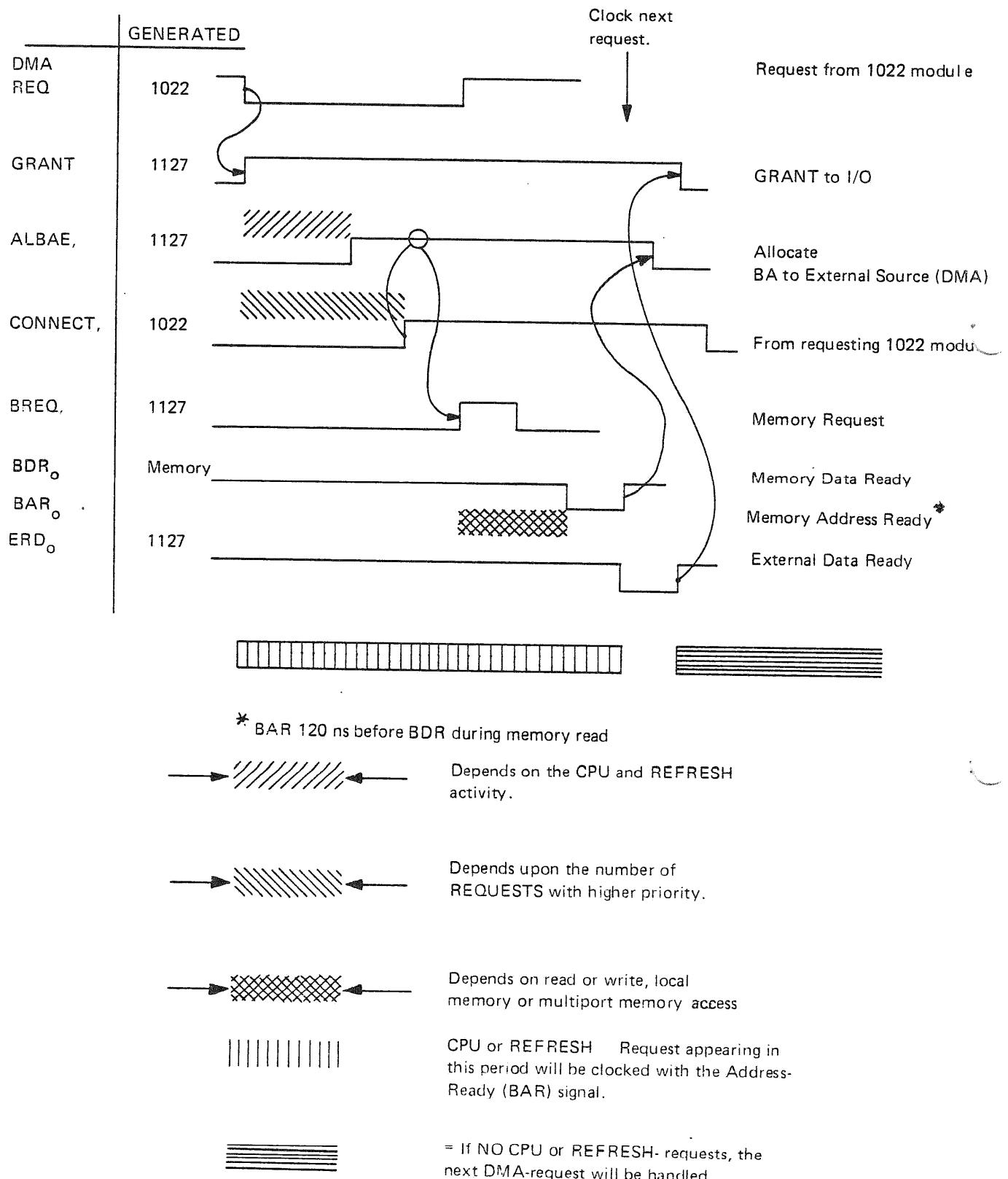
Figure 6.9: DMA TIMING DIAGRAMS:
