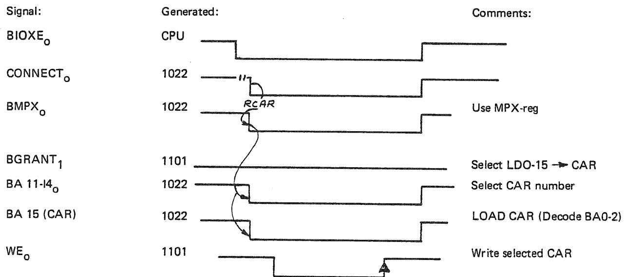
**2. INCREMENT MPX-CAR during DMA**
