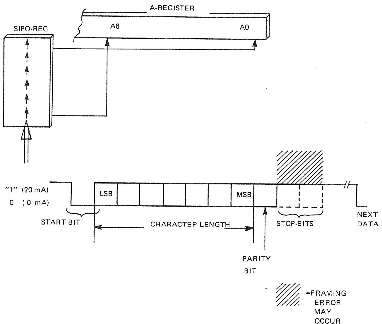
Figure 2.1: ASCII SERIAL FORMAT
