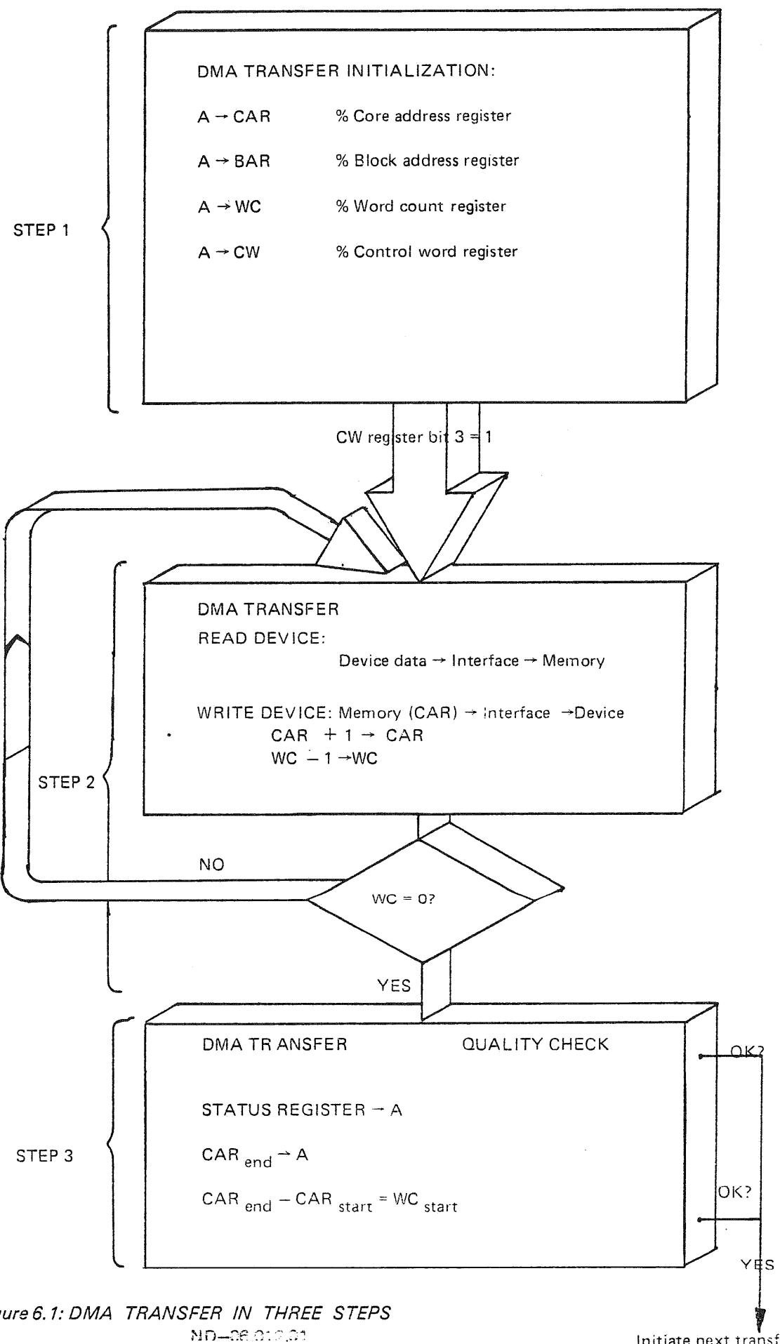
Figure 6.1: DMA TRANSFER IN THREE STEPS
