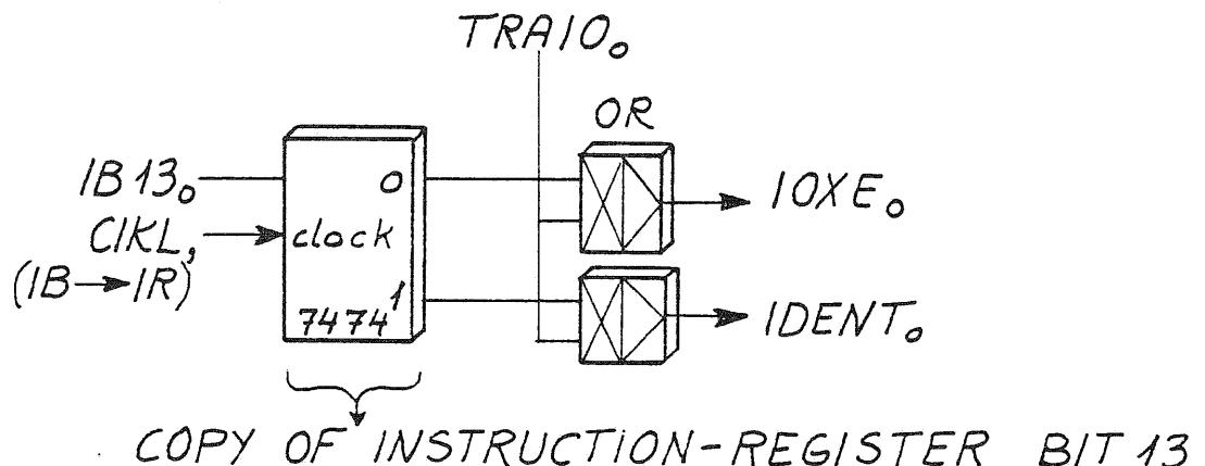
Figure 4.2: IOXE/IDENT SIGNAL GENERATION
