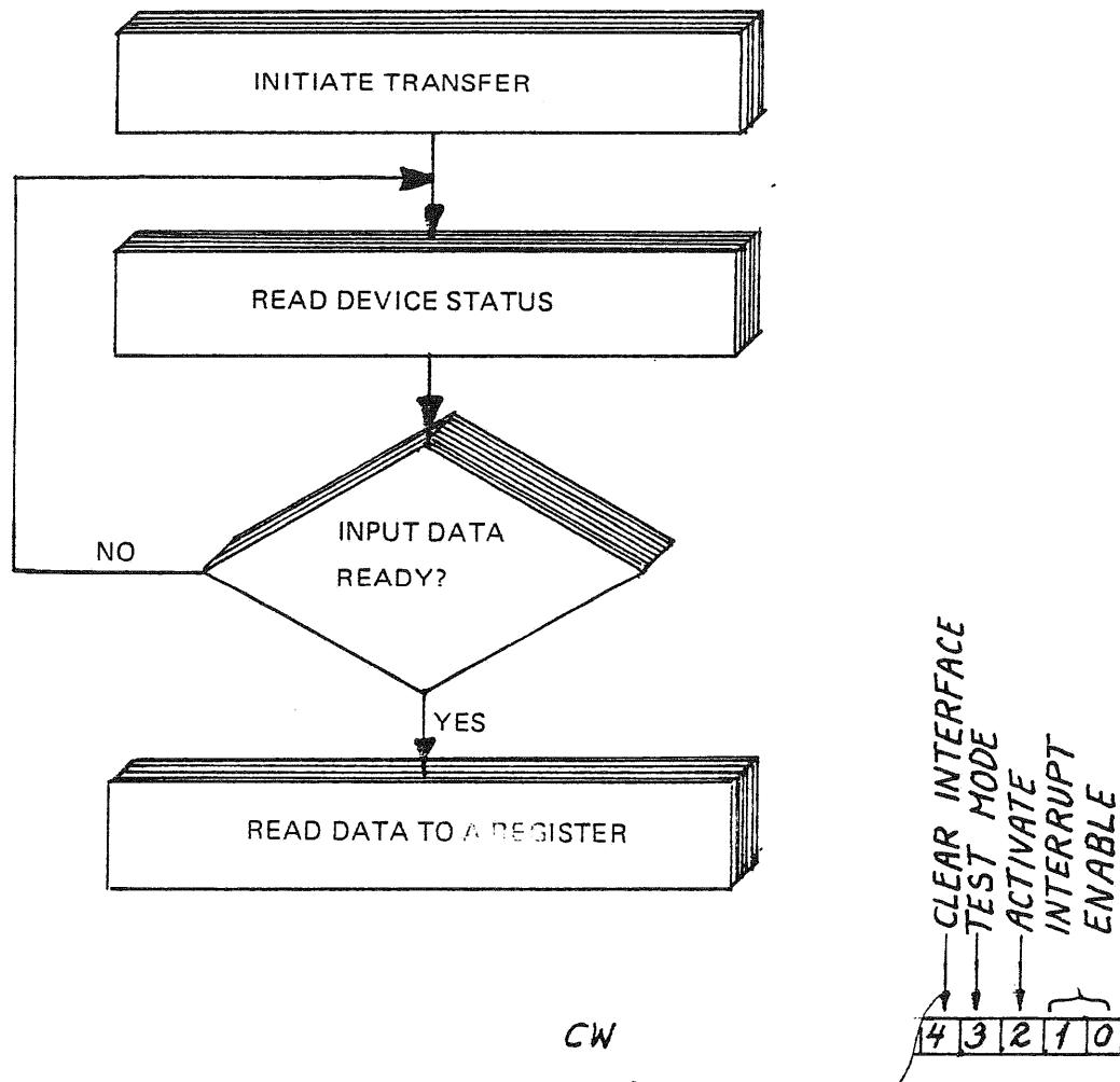
The transfer is initiated by setting the CONTROL-WORD REGISTER informing of:
